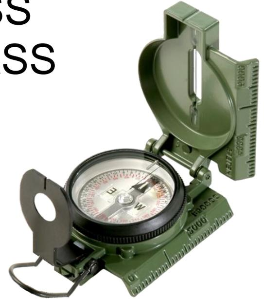
EFFECTS OF METAL AND ELECTRICITY – these sources affect the performance of a compass during use.
